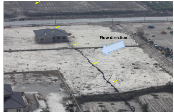
Figure 4: Aerial view of the northern section of the crack (courtesy of Puerto Lumbreras City Council). The yellow arrows indicate the location of the earth fissure. Modified from Mulas (2013).
