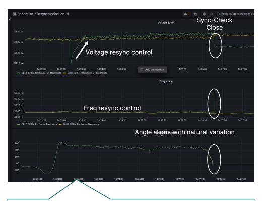
Resync boundary VF $\delta$  differences to align
