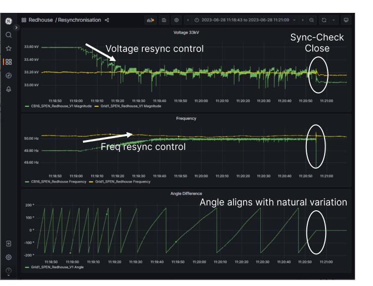
Resync Control Mode brings zone voltage and frequency into alignment with external grid through P&Q setpoint control, shifting position on droop line.
