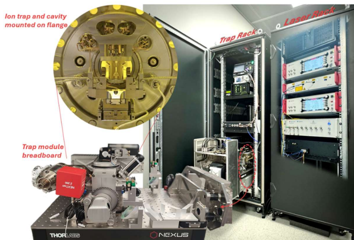
Figure 55: Quantum network processing node with rack-mounted ion-trap cavity system.
