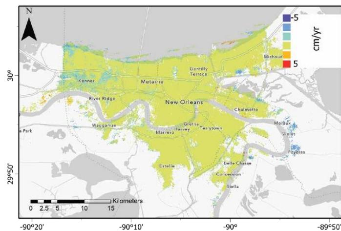
Figure 1 Subsidence rates from 4 years of InSAR data [Jan. 2018 – Dec. 2021] for the area around the city of New Orleans. Most of the urban area is stable except for some subsidence in the Michoud area.
