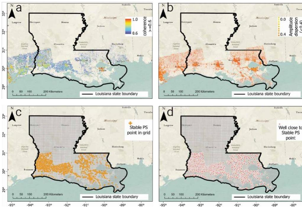
Figure 2 Location of InSAR (a) spatial coherence exceeding 0.6 and (b) amplitude dispersion below 0.4 for four Sentinel-1 SAR scenes over Southern Louisiana. (c) Points of stable InSAR return in each of uniformly divided 5kmx5km grids and (d) the location of the closest abandoned oil well site.
