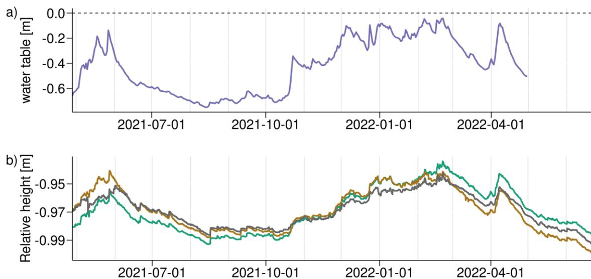
Figure 2 a) Water table and b) relative surface heights measured with three extensometers.
