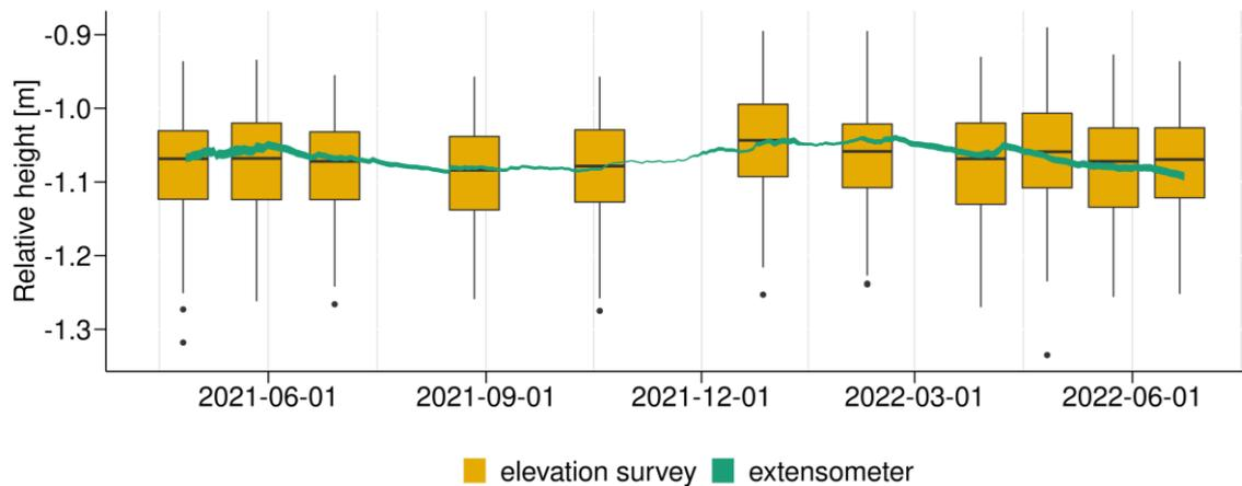
Figure 3 Extensometer measurements (standard deviation of three extensometer) and repeated elevation surveys (boxes define the 25-75% quartiles, whiskers are 1.5 times the quartile, points represent values outside this interval).
