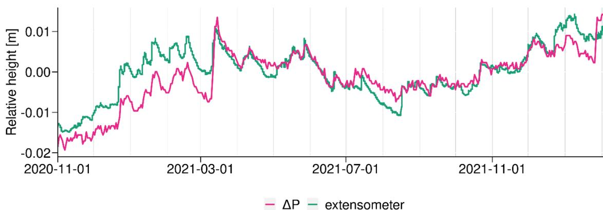
Figure 1 Relative heights measured with an extensometer and a 'fixed' and 'moving' pressure transducer ( $\Delta P$ ).
