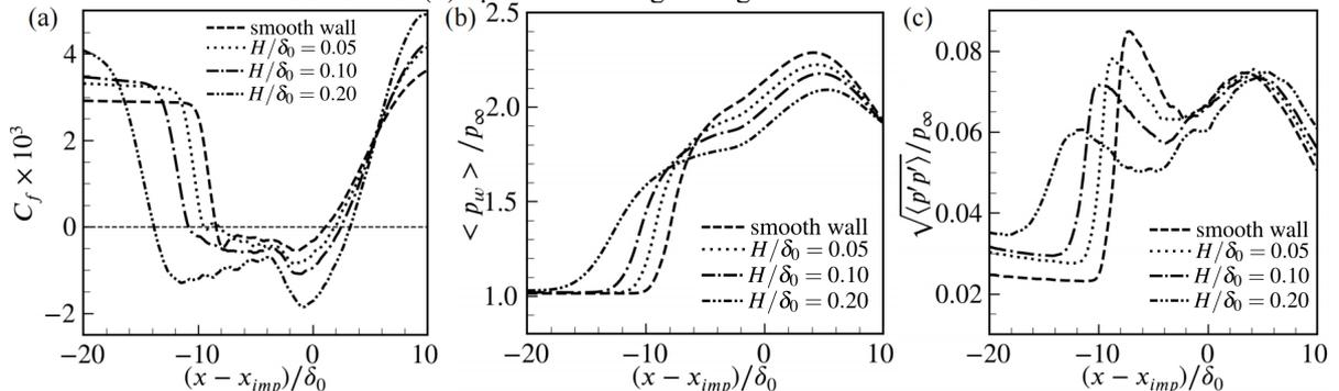
Figure 3. Spanwise averaged (a) wall pressure and (b) wall pressure fluctuations (c) friction coefficient for smooth wall.
