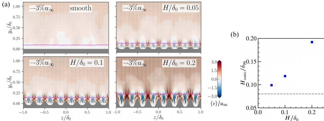
Figure 2. (a) Vertical velocity in a cross-stream plane with superposed cross-stream velocity vectors. The solid line shows the sonic line. (b) Spanwise-averaged height of the mean sonic line.
