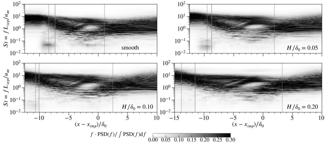
Figure 4. Pre-multiplied power spectra density maps of wall pressure signals at the mid-plane. The dotted lines denote  $C_f=0$ ; the solid lines denote the location of maximum pressure fluctuation.
