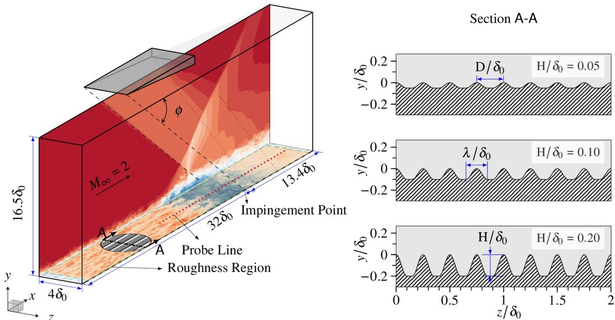
Figure 1. (a) Schematics of the computational domain (including streamwise velocity contours), and (b) schematic view of the investigated ridge-type rough walls with relevant definitions.
