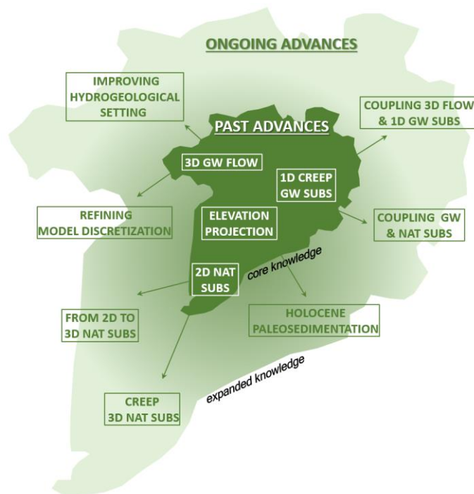
Figure 3 Past and ongoing advances in numerical modelling of subsidence in the Mekong. The modelling advances encompass both natural (NAT) and groundwater (GW) extraction-induced subsidence (SUBS), processes acting in different depth domains under different drivers.
