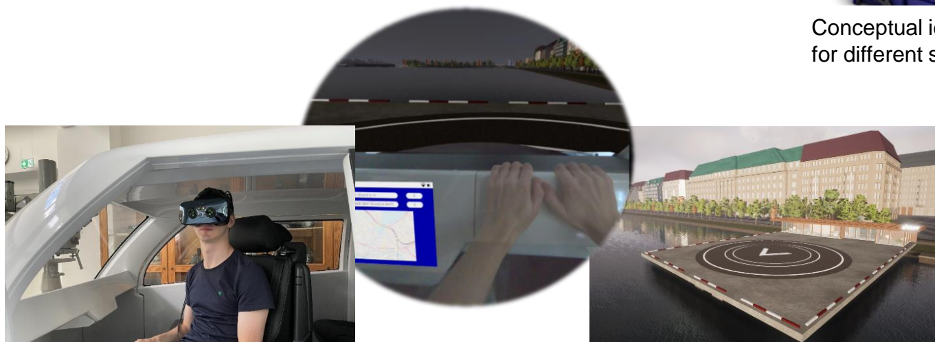
Simulator set-up with cabin mock-up and head-worn mixed reality display, virtual Hamburg scenery
