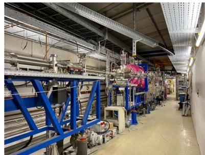
Figure 5: Schematic of the HITRAP facility in the frame of the GSI accelerator (left). Picture of the decelerator beamline (right).
