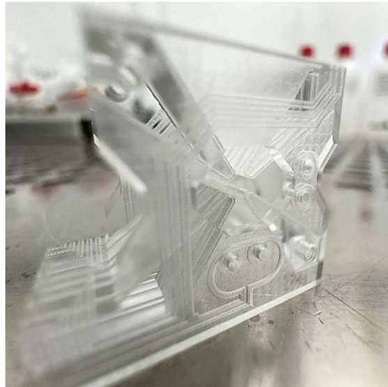
Figure 19: 3D ion trap blank made from a piece of fused silica using SLE.
