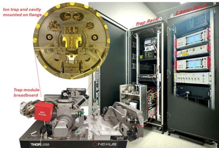
Figure 51: Quantum network processing node with rack-mounted ion-trap cavity system.
