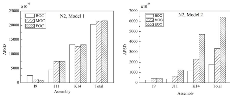
Figure 4: APSD (a.u.) of ex-core detector induced by simultaneous stochastic vibrations of fuel assemblies J9, K11 and L14 in a PWR.
