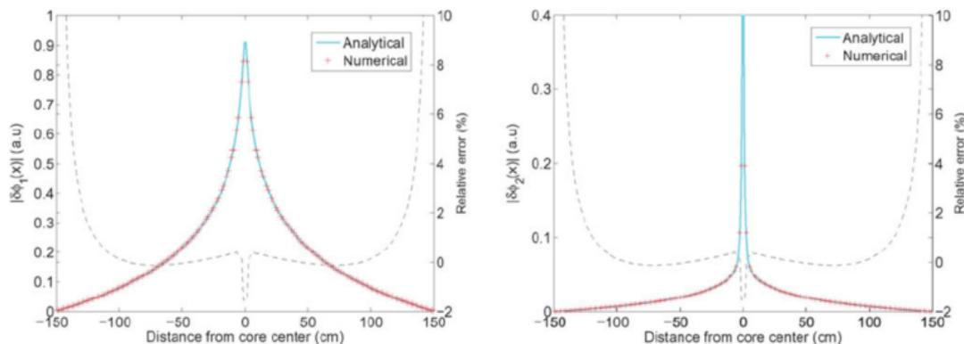
Figure 1: Comparison of fast and thermal noise in a PWR between numerical and analytic calculations.
