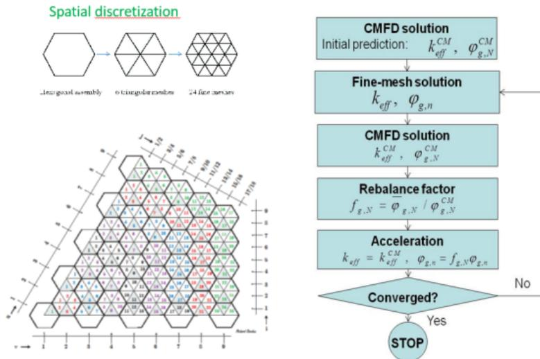
Figure 6: Triangular discretization and flowchart of noise solution for hexagonal
