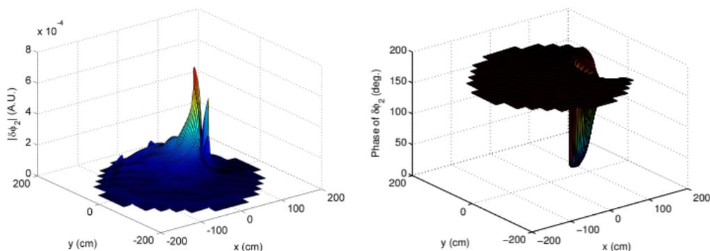
Figure 3: Magnitude and phase of thermal noise induced by trajectory vibration of assembly M10 in xy-direction ( $f = 8$  Hz).
