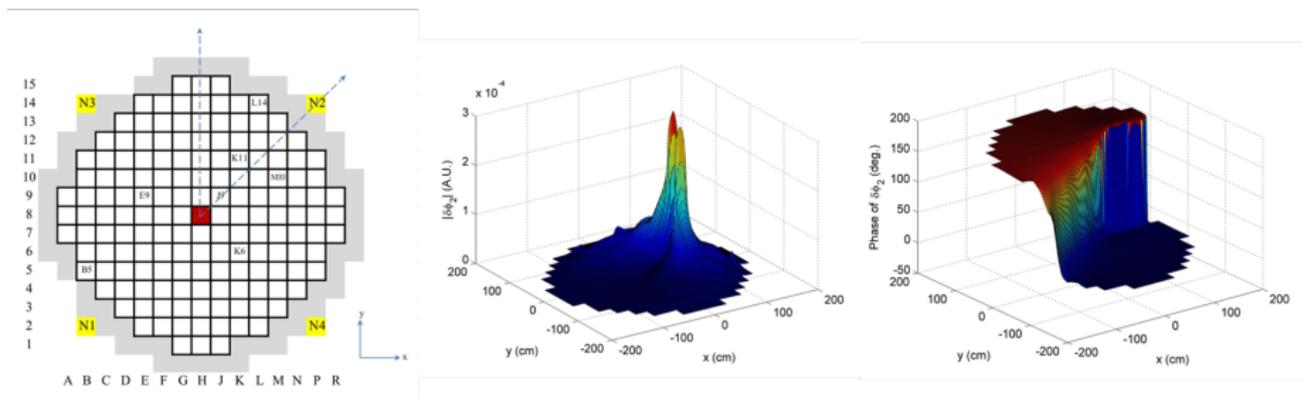
Figure 2: Magnitude and phase of thermal noise induced by vibration of assembly M10 in x-direction ( $f = 8\text{Hz}$ ).
