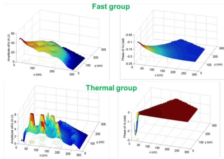
Figure 9: Amplitude and phase of space-dependent noise in fast (group 9) and epi-thermal (group 20) groups ( $f = 1\text{Hz}$ ).
