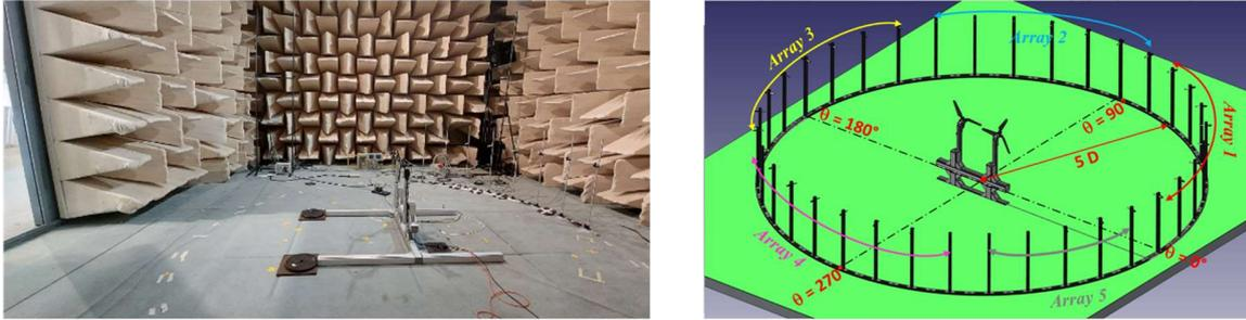
Figure 5: Experimental setup diagram inside the anechoic chamber. The circumference on which the microphones were positioned and the definition of the polar angle  $\Theta$  are also shown.
