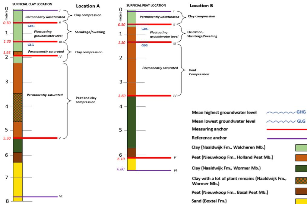
Figure 3 Schematic overview of the lithological build-up and the two extensometer sequences (in meters below the land surface), with their anchor positions and corresponding measuring purposes. The surface level of the surficial clay location is elevated 1.48 m below mean sea level. The surface level of the surficial peat location is elevated 2.40 m below mean sea level.
