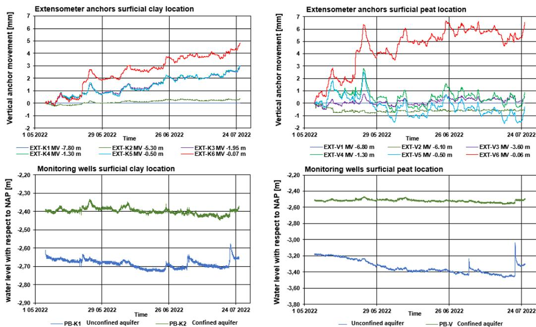
Figure 4 First extensometer results and groundwater level results. Vertical anchor movements in meters are with respect to the original measurement. Anchor positions are with respect to the surface level which is respectively 1.48 m below the mean sea level for location A with surficial clay and 2.40 m below mean sea level for location B with surficial peat.
