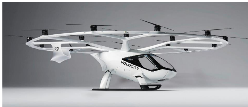
Figure 3: VoloCity with two passengers and 11.3 m maximum distance (picture taken from 2021 white paper [24]).
