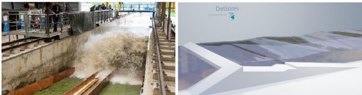
Figure 3: Wide Green Dike under wave attack. Left: Physical flume. Right: Numerical flume.
