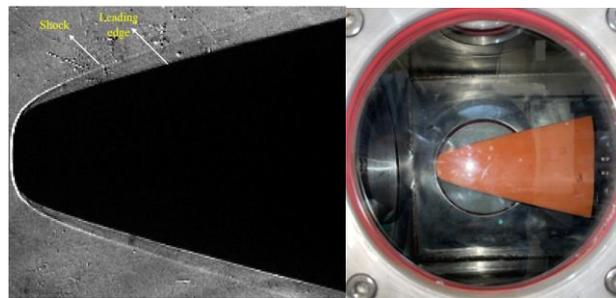
Figure 2: On the right is the plan view of the mounted waverider model, with its corresponding schlieren image displayed on the left at 0° Angle of Attack.
