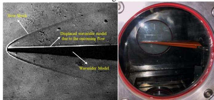
Figure 3: On the right is the side view of the mounted waverider model, with its corresponding schlieren image displayed on the left at 0° Angle of Attack.
