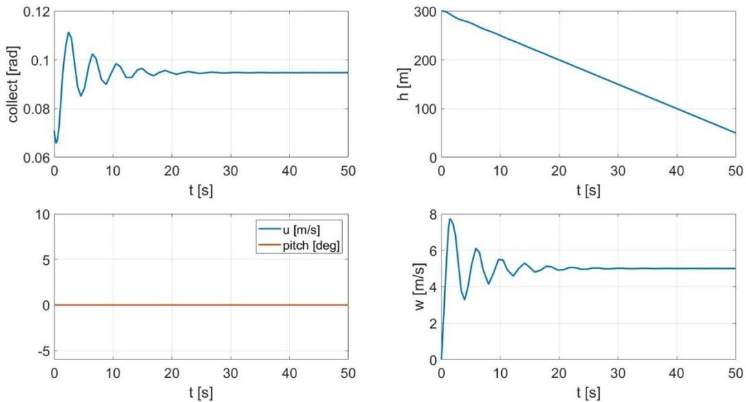
Figure 16: Rate of climb control upper mode without Avoidance System.
