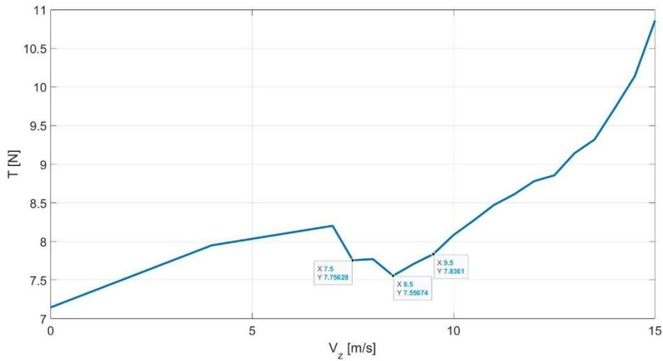
Figure 9: Load cell data that highlight the thrust (N) drop.
