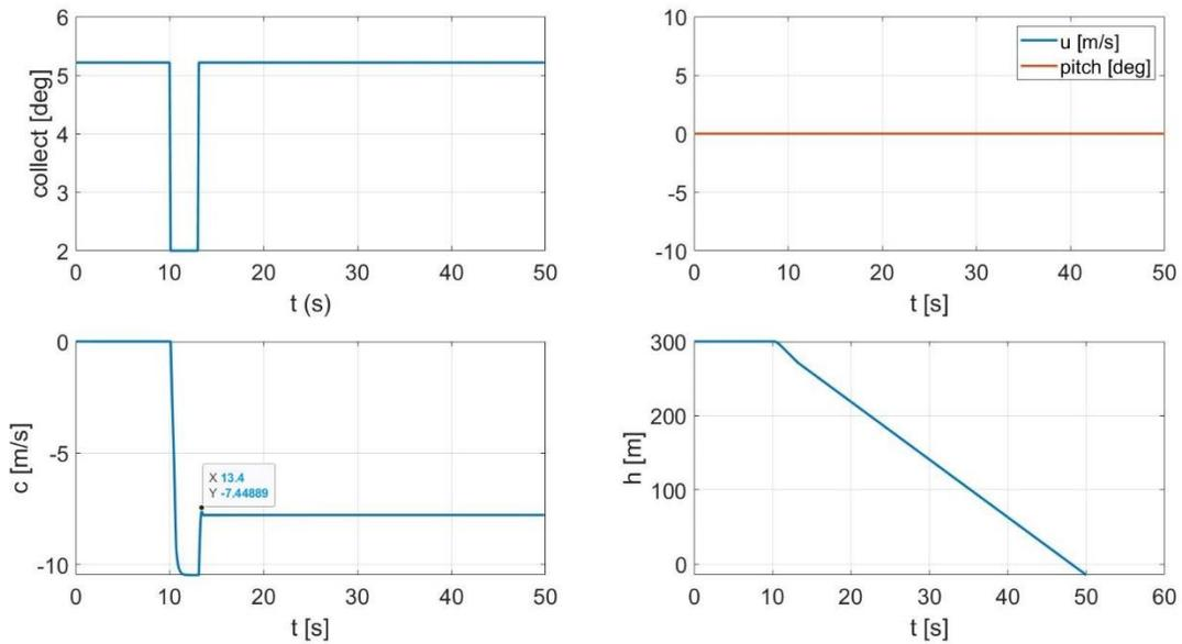
Figure 12: Flow model with Vortex Ring State simulation results.
