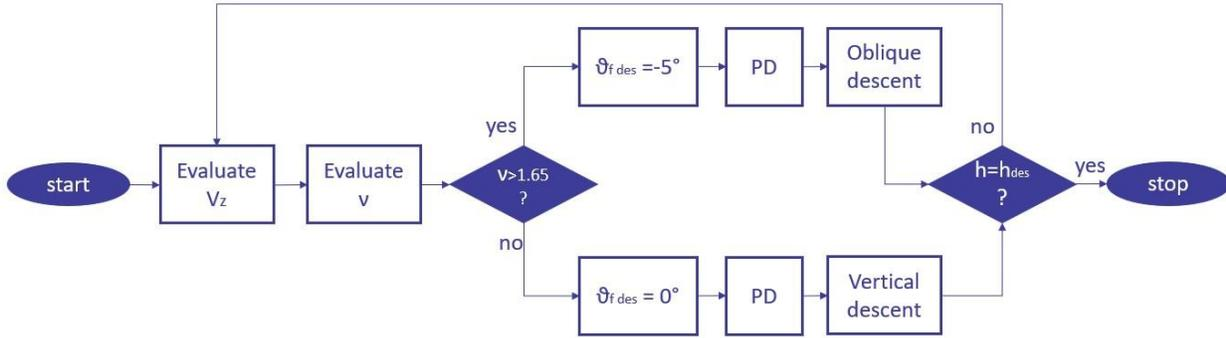
Figure 10: VRS Avoidance System function logic while altitude control is engaged.
