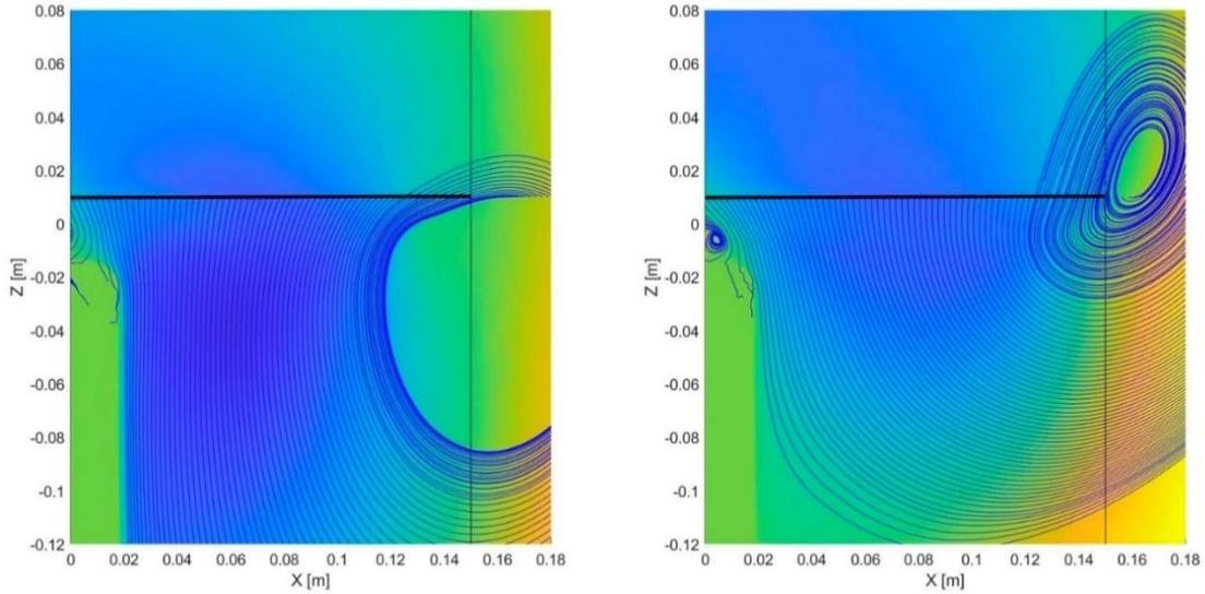
Figure 6: PIV results at Vz 8.5 m/s and 9.5 m/s.
