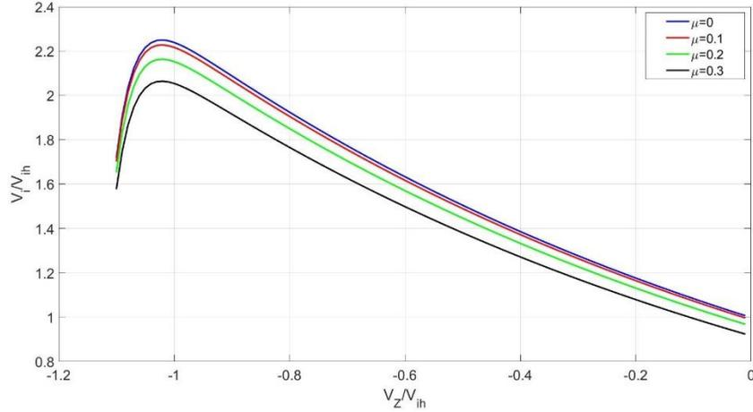
Figure 8: Induced velocity model with Vortex Ring changing the forward speed.
