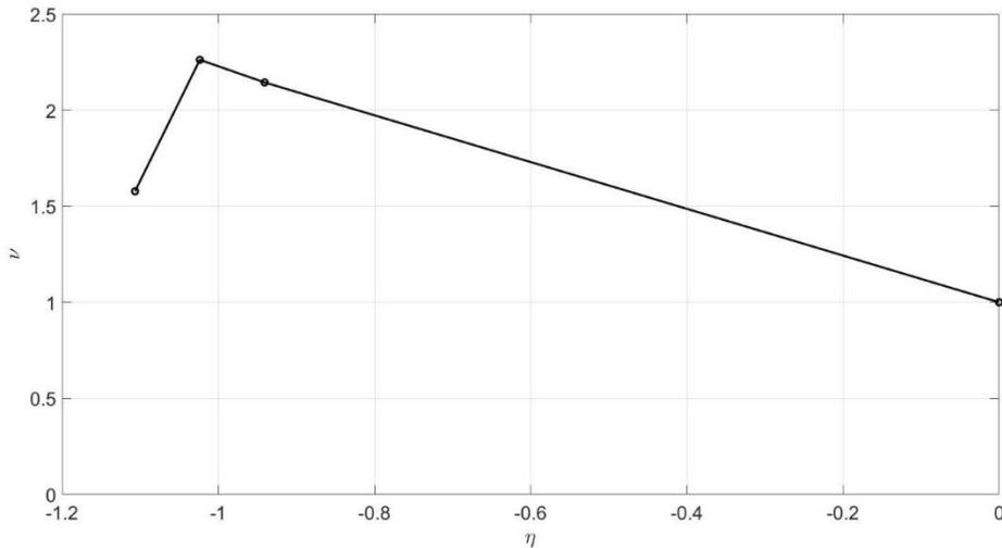
Figure 7: Induced velocity in VRS state [4]
