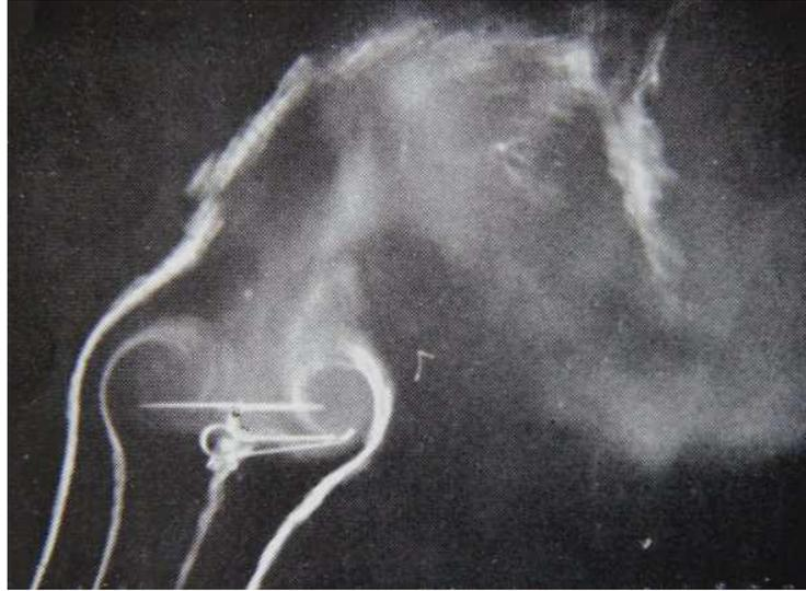
Figure 3 Smoke visualisation of helicopter rotor in vortex ring state [6]
