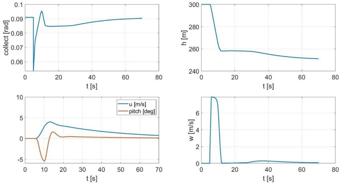
Figure 14: Altitude control upper mode with Avoidance System active.
