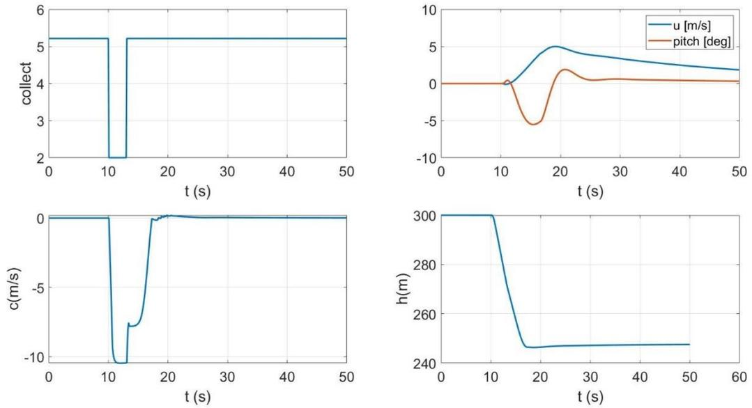
Figure 13: Flow model with Vortex Ring State and Avoidance System simulation results.
