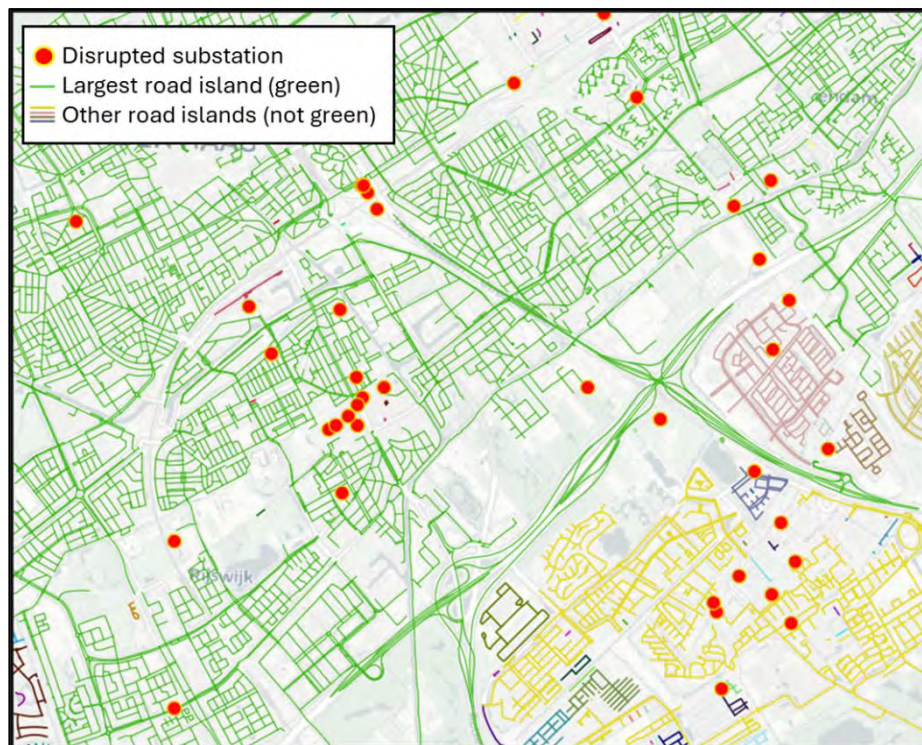
Figure 3. Disrupted substations in the southeastern area of The Hague and isolated sections of the road network (islands) in different colours; the largest connected component is coloured green. Transit between sections of the road network of different colours is not possible due to flooding.
