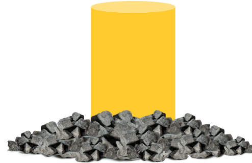
Adjust scour protection (e.g. shape, dimensions) to provide settlement habitat
