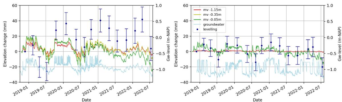
Figure 2 Extensometer (three measurement levels), levelling (average with standard deviation indicated by vertical bars) and phreatic groundwater monitoring results for locations 05-REF (left) and 09-REF (right). Elevation changes measured by the extensometers are relative to October '18, for levelling relative to November '18.
