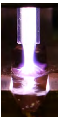
Fig.1. Surface-wave microwave discharge in contact with water flowing in a 9 mm trapezoid channel.
