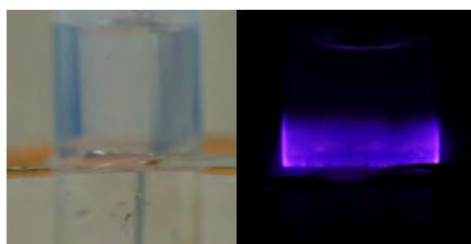
Figure 1. Surface Dielectric Barrier Discharge with liquid electrodes.
