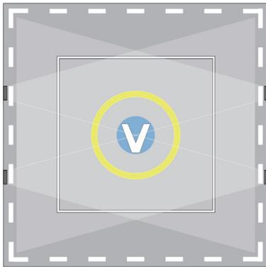
Figure 1: Example of a rectangular FATO and TLOF, from [6]
