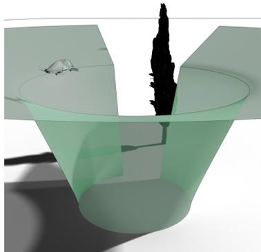
Figure 2: Example of a conical OFV with omnidirectional approach and take-off climb surface and prohibited sector, from [6]
