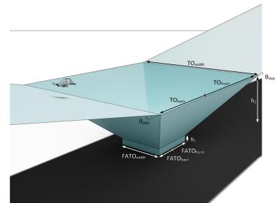
Figure 3: Vertical take-off and landing procedure volume and its defining parameters, from [6]
