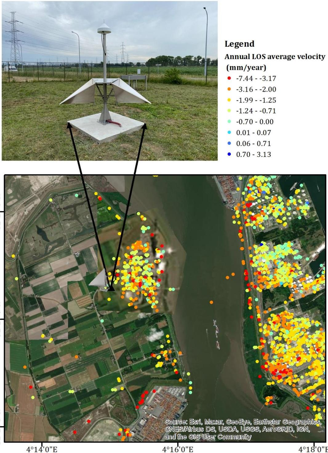
Figure 1 Location of installed IGRS on the average annual velocity map of the PS points calculated from applying PS-InSAR on Sentinel-1 radar data
